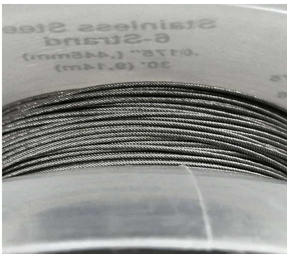
شکل ۳- 0/0175 stainless steel 6-strand Coaxial wire
