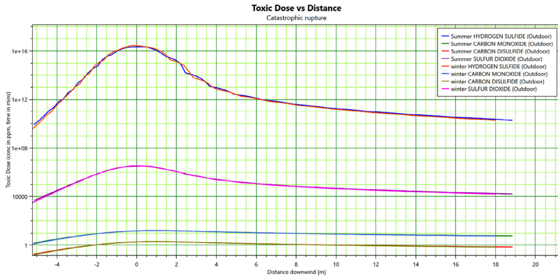
Fig. 4: Toxic dose vs. distance in wind direction for Catastrophic Rupture scenario
